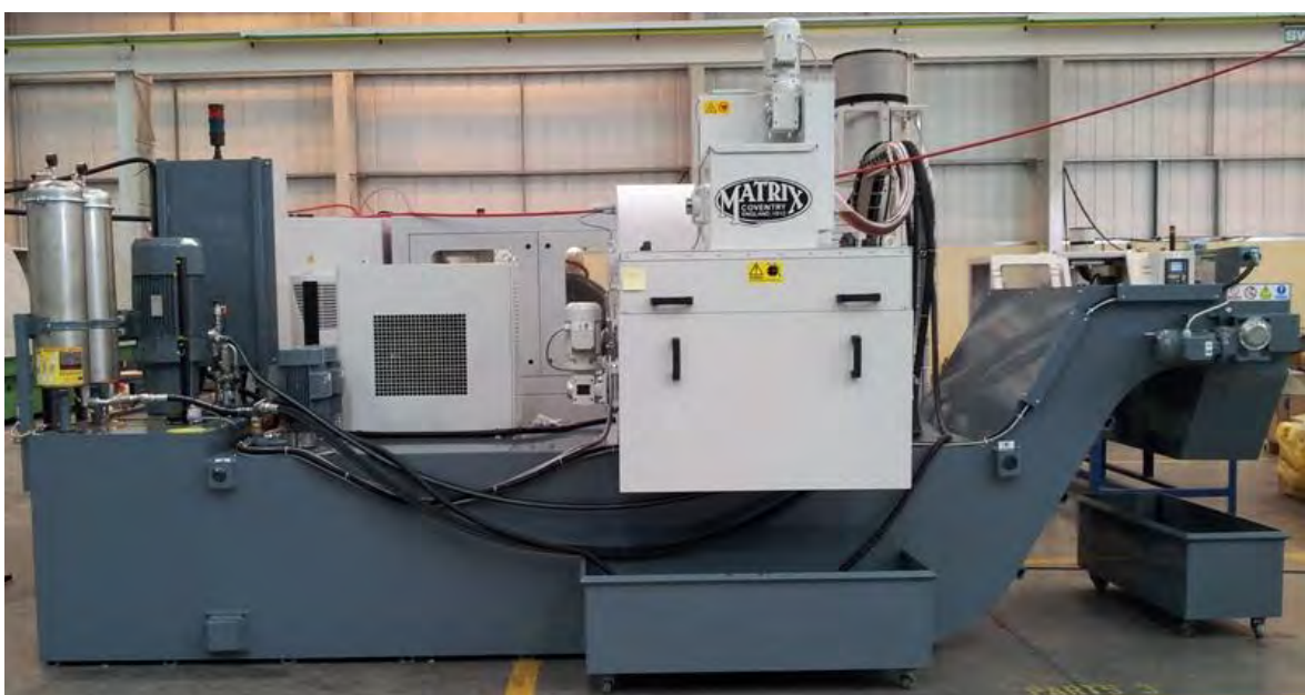
Coolant system view (rear of machine)
