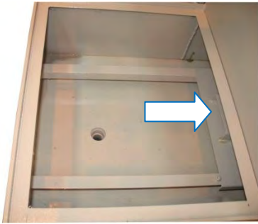
Catch plate shown in the normal operating position
