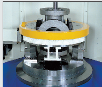
Automatic Index Chuck (for machining small valve)
